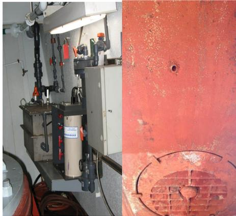
Fig. 1. Sea temperature instrumentation for the TG THOMPSON. Here, we have (a) internal thermosalinograph, and (b) intake sensor (located near the small hole in the upper half of the image).
